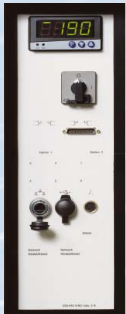
Main switch, test specimen protection and interfaces
