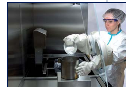
Laminar flow clean air system for product protection in filling of pharmaceutical products
