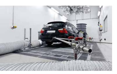
In addition, it permits sunlight simulation at up to 1000 W/m<sup>2</sup>. On the test bench, an airstream blower creates wind with a velocity of up to 120 km/h, proportional to the simulated driving speed.
