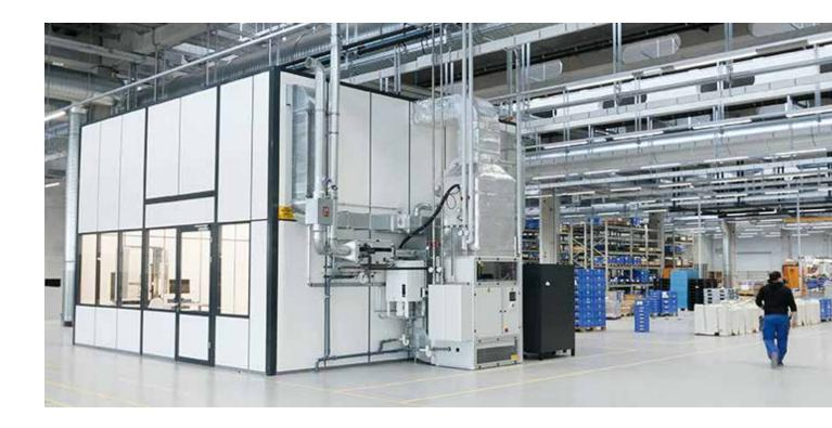
checks supplier's parts for dimensional accuracy. The second measuring room is concerned with quality assurance during and at the end of the in-house manufacturing process. "Some of the manufacturing tolerances to be measured are about one  $\mu$ ," says Jörn Winkler.
