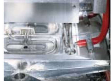
Wet-bulb thermometer with forced humidification
