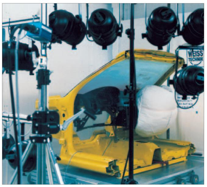
Airbag Testing System for Research and Quality Assurance The system comprises the temperature conditioning chamber, a sliding test frame with runners, automatically closing gate and switch cabinet with control system. The testing system is for testing the performance of airbags at extreme temperatures.
